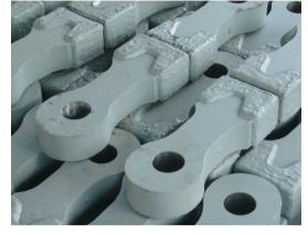
Heavy duty vertical shredder prepares the cane before sugar extraction. It conditions the energetic performance of the whole plant and maximizes sucrose recovery.
